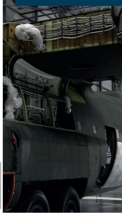
Marshall is the only Maintenance, Repair and Overhaul organisation outside of the USA capable of replacing the Centre Wing Box (CWB) on both legacy C-130 and C-130J, providing valuable aircraft life extension.
